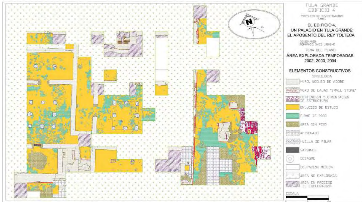
Figure 10. The explored area and the state of conservation of constructive elements in Building Four.
