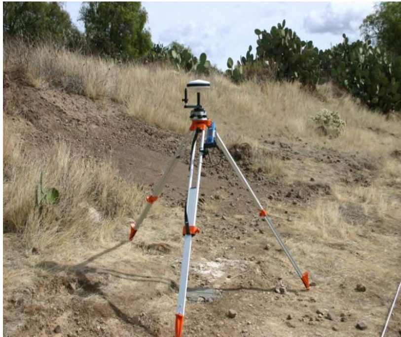
Photo 7. Measuring coordinates with Global GPS.
